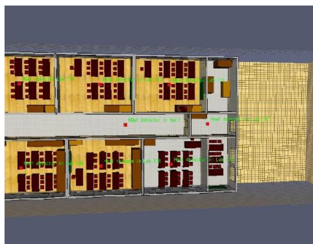
Figure 7 - Simulation model of the second floor of the Electro technical school “Nikola Tesla” laboratory part, with positioned heat detectors (above view)
