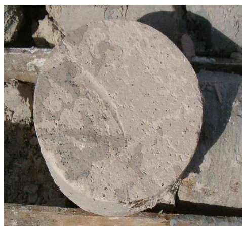
Figure 7 - Cross-section through the core of “solid and compact” ash layer
