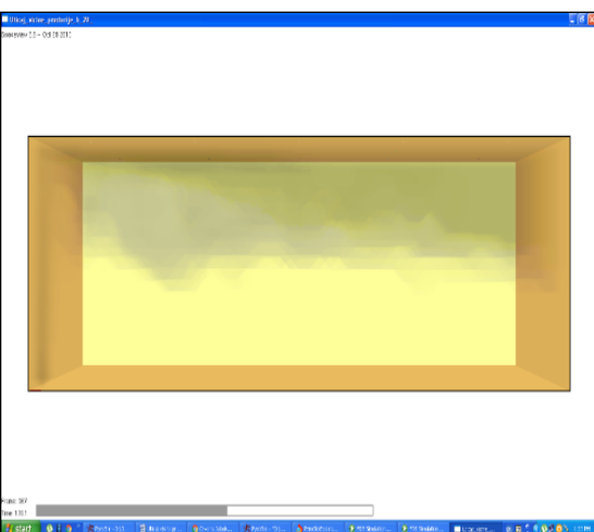
Figure 32 - Smoke propagation in simulated object for burner with HRR of 1500 kW/m 2 and room's height of 30 m after 170.5 seconds
