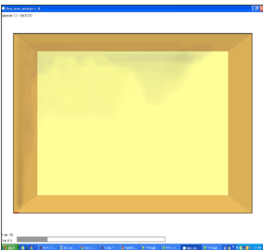
Figure 31 - Smoke propagation in simulated object for burner with HRR of 1500 kW/m 2 and room's height of 30 m after 61.8 seconds
