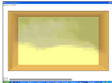
Figure 4 - Smoke density decrement with height for simulation model of room with 30m height (front view)
