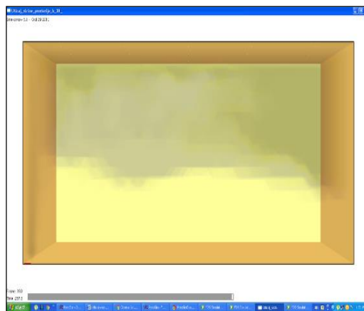
Figure 33 - Smoke propagation in simulated object for burner with HRR of 1500 kW/m 2 and room's height of 30 m after 297.9 seconds
