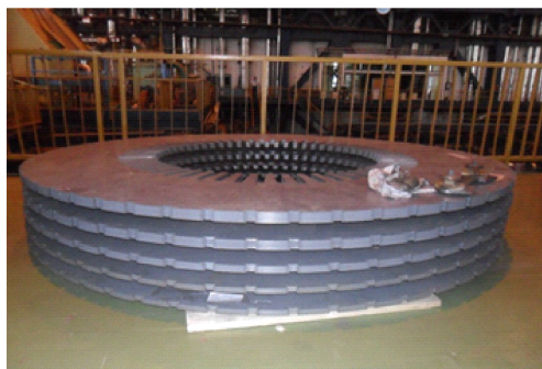
Figure 2. Monolithic packs for replacement of the end part of stator magnetic core for turbogenerator n.1 in TPP Bitola
