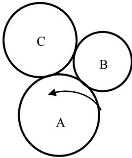
*Figure 1. Necessity of sliding in a cluster of particles. The centers of three particles A, B and C are fixed and the particles are in contact with each other. Impose the counterclockwise rotation on particle A, as shown. Relative sliding is defined by non-zero relative velocities of the contact points. To avoid sliding with respect to A, both B and C must both rotate in the clockwise direction. But this will result in sliding on the B-C contact.*
