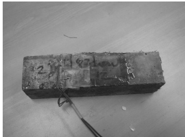
b) Electrical-resistant gauge for measuring the deformation in the tensile zone
