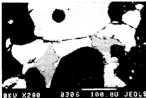
Fig. 1. Distribution of magnetite and ilmenite in ore materials; white-magnetite; greyilmenite; black-silicate minerals*
