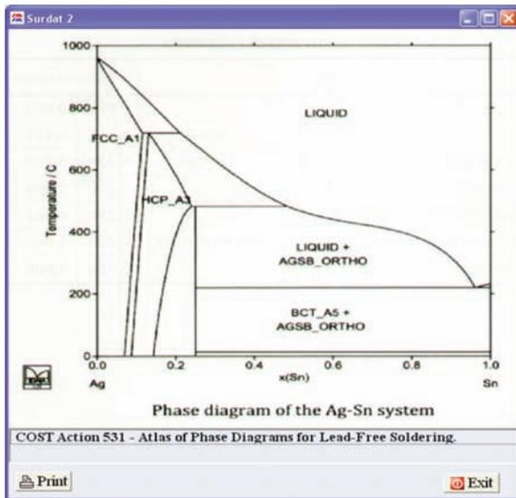
Figure 3. Phase diagram of the Ag-Sn system [9].
