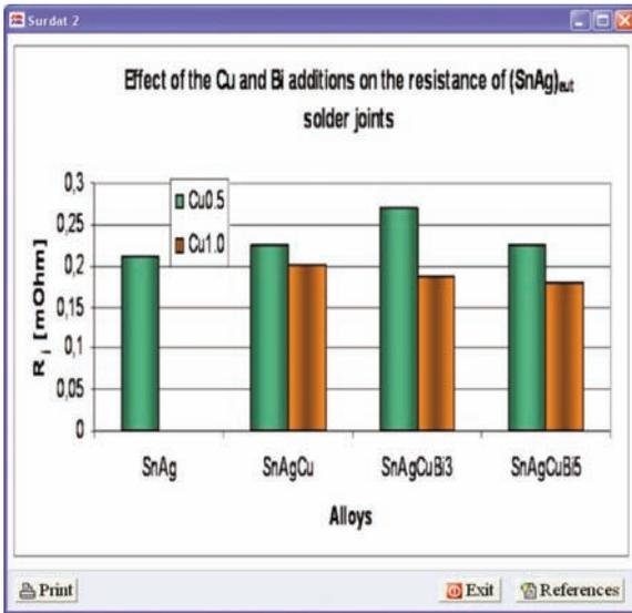
Figure 6. Influence of Cu and Bi additions at the resistivity of (SnAg)<sub>eut</sub> lead-free solders.
