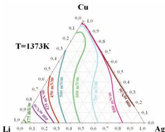
Figure 9. Isolines of the surface tension in Ag-Cu-Li system at 1373K.
