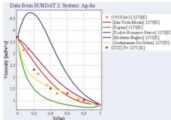
Figure 8. Isotherms of viscosity calculated by different models compared with the experimental data of Gebhardt et al. [10] [1953Geb1] together with the hypothetical XYZ data at 1273 K.
