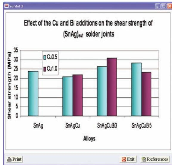
Figure 7. Influence of Cu and Bi additions the (SnAg)<sub>eut</sub> lead-free solders.
