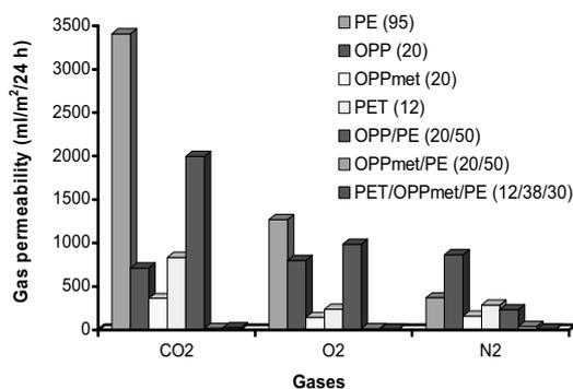
**Fig. 2.** Gas permeability of different packaging materials
