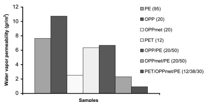
**Fig. 3.** Water vapour permeability of different packaging materials
