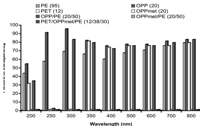
**Fig. 1.** Permeability of light in different packaging materials
