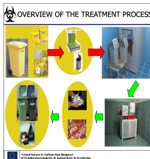
Figure 4 - Overview of the infectious healthcare waste treatment process
