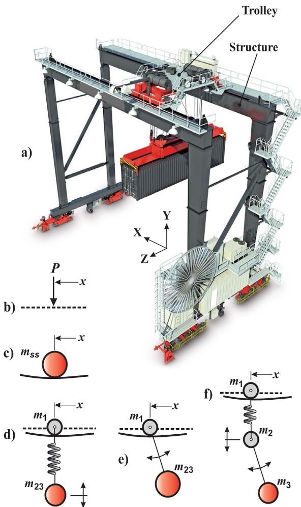
Figure 1. a) RMG container crane, b) Moving force (MFM), c) Moving mass (MMM), d) Moving oscillator (MOM), e) Moving pendulum (MPM), f) Moving oscillator with pendulum (MOPM).
