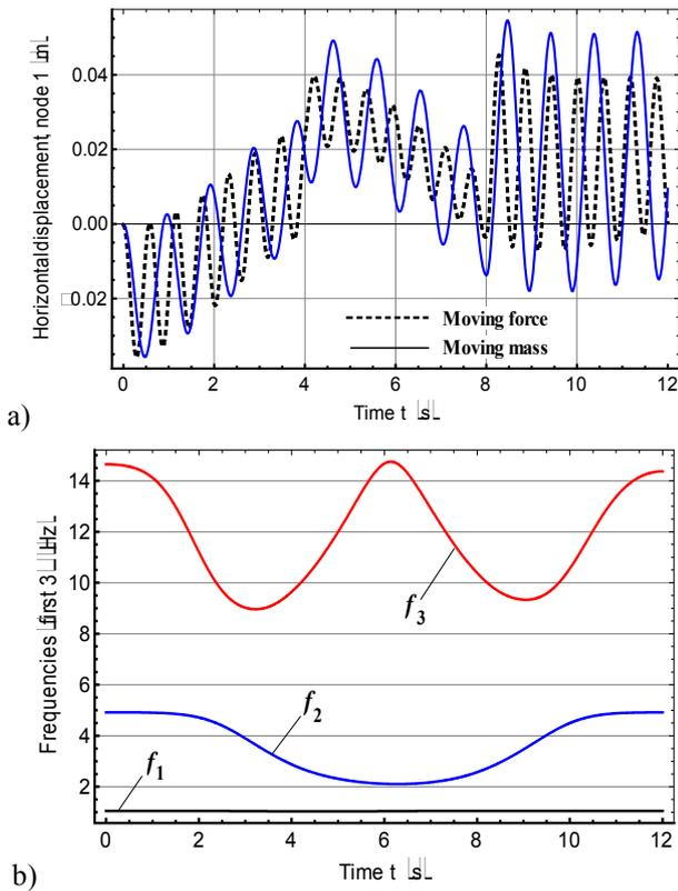
Figure 4: a) MMM/FFM Horizontal displacement  $U_{x1}$ ,  $v_2$ , b) MMM first 3 frequencies
