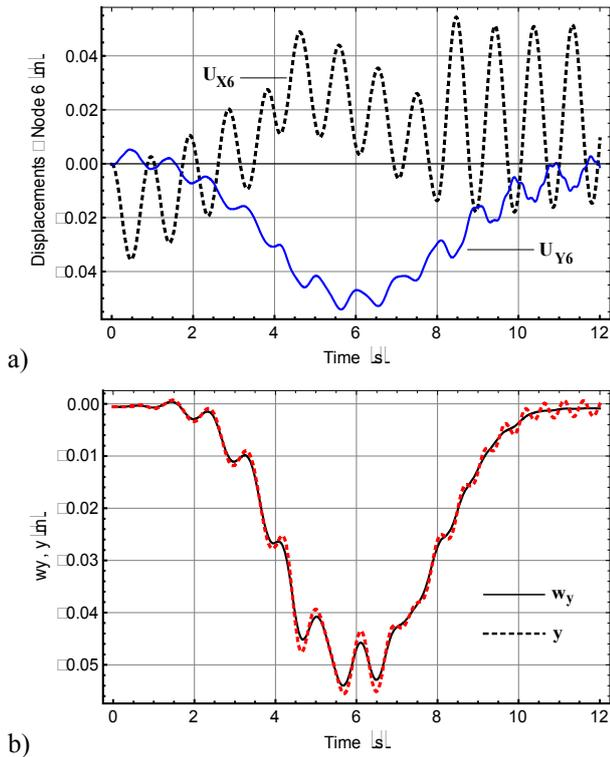
Figure 5: MOM, a) Vertical and horizontal displacement-node 6, b) Displacement  $y$ ,  $k=10^7$  N/m;  $v_2$ .
