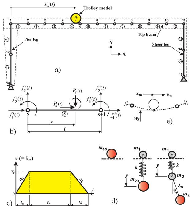
Figure 2: a) FE model of the gantry crane structure, b) Equivalent nodal forces of the elements  $s$ , c) Speed pattern of the moving load, d) Moving load models - MMM, MOM and MOPM, e) Contact point displacements.
