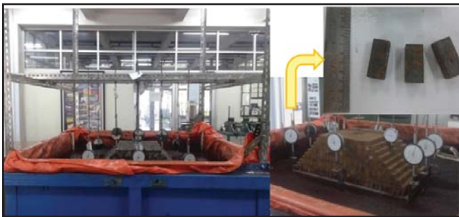
Figure 2: Laboratory small-scale model for embankment load test
