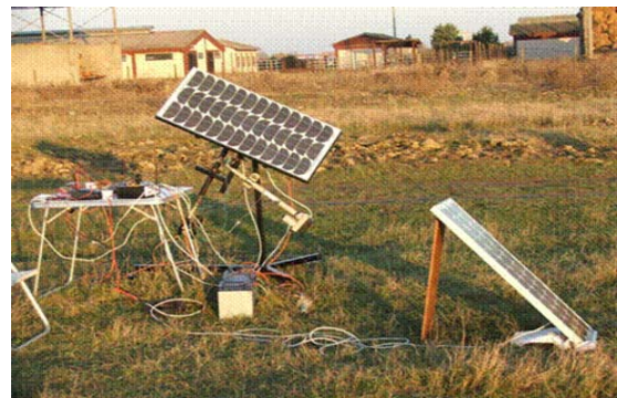
Fig. 8. Experimental two-axis solar tracker
