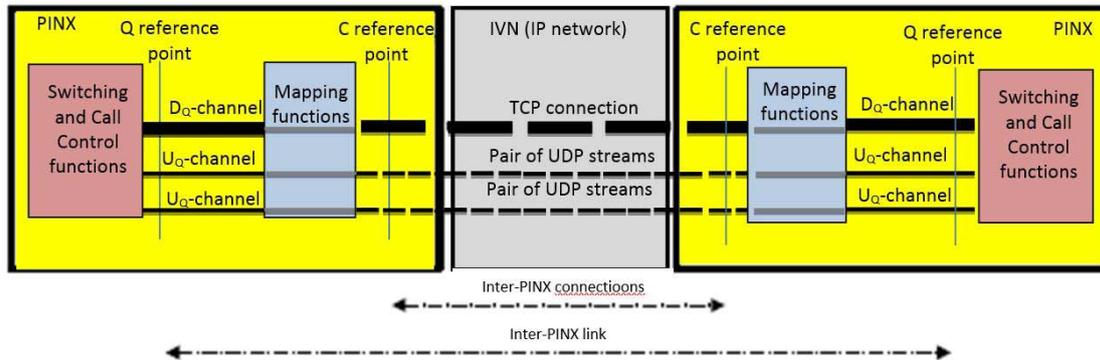
**Figure 5.** IPC concept for "Semi-permanent" TCP connection (Ecma International, 2002)
