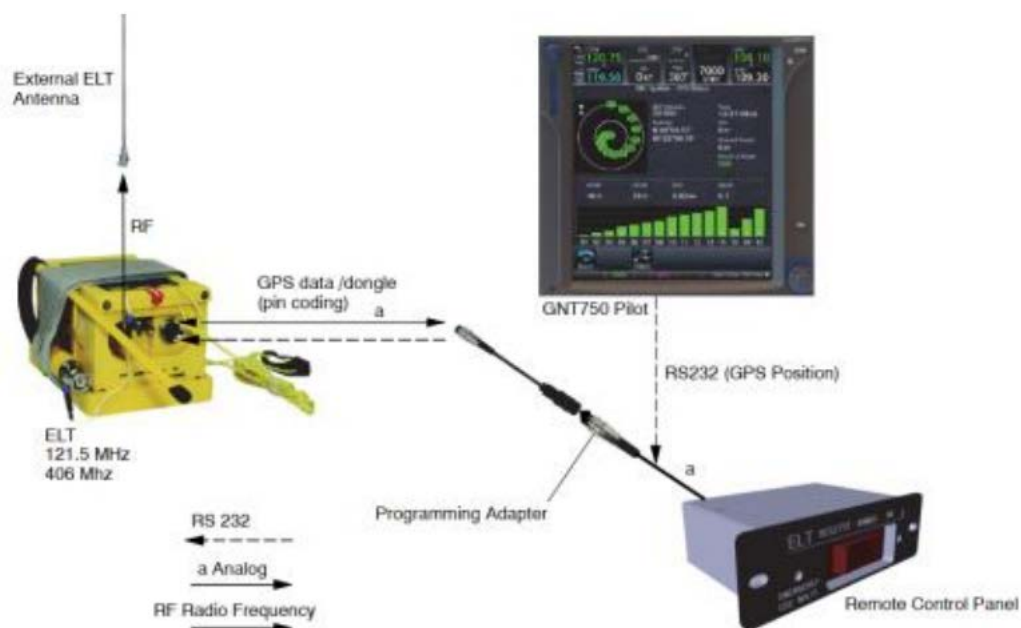
Figure 4 – Components of the ELT device
