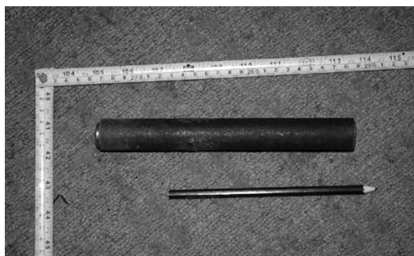
Figure 2. Iron tube lying on the floor, approximately 22 cm long, about 3 cm in diameter, with hunting cartridge inserted
