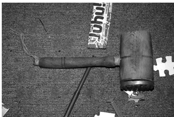
Figure 3. Wooden hammer that has a thick metal plate with many small cone-shaped wedges
