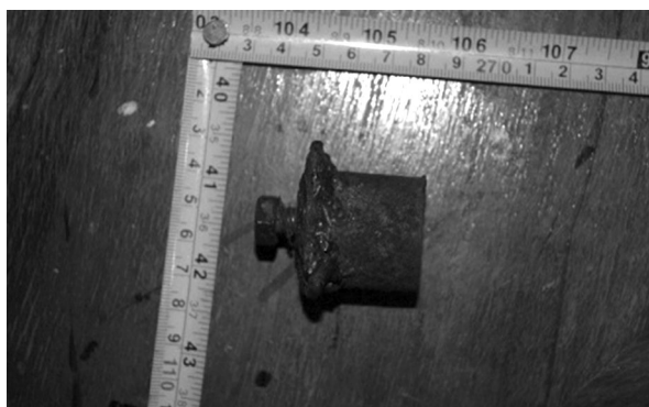
Figure 4. Small cylinder closed with a rectangular plate, screw breaching through the plate and ending with a spike used as a firing pin
