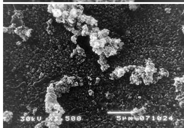
Figure 7. SEM: Typical appearance of self-nucleated CHA, after 33 days nucleation in mixture solution of supersaturated SBF and FCS.
