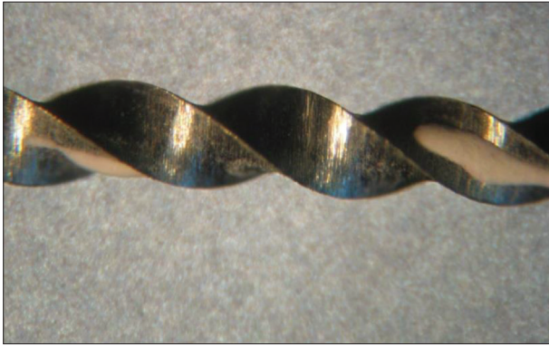
Figure 4. Residual deposits of calcium hydroxide on a size 35 file, after treatment with an enzymatic cleaner (grade 3)
