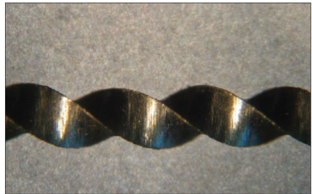
Figure 7. Clean instrument surface without calcium hydroxide deposits subjected to the combined decontamination method
