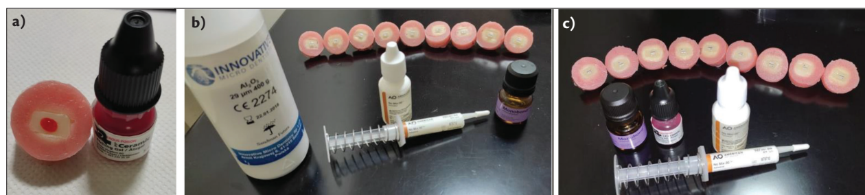
Figure 2. a) Etching the samples with 4% HFA; b) Prepared samples from group 4; c) Prepared samples from group 5
