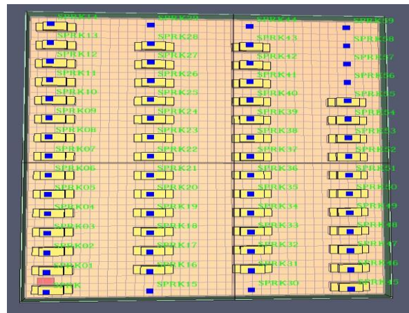
Figure 11 - 3 D simulation model with the drencher nozzles arrangement of the auto garage and burner's position at the corner of the garage
