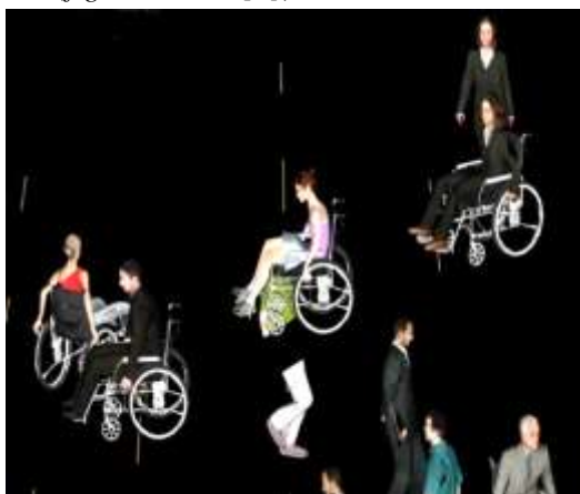
Figure 10 - The evacuation moment for the scenario I (the mobile occupants/patient's speed 1.5 m/s, wheelchairs speed 0.69 m/s)
