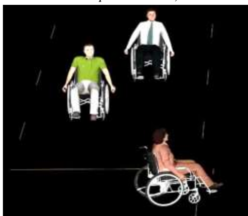
Figure 11 - The evacuation moment for the scenario V (the mobile occupants/patient's speed 2 m/s, wheelchairs speed 0.69 m/s)
