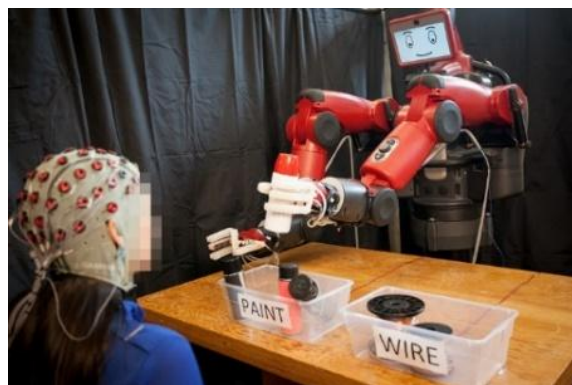
Figure 10 - The feedback system enables human operators to correct the robot's choice in real time. After [127]
