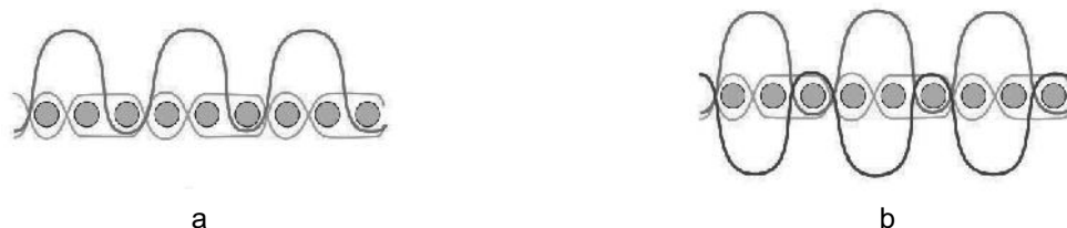
Figure 1: Cross-section of terry fabric: a – with single pile (loops on one side); b – with double pile (loops on both sides)
