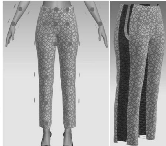
Figure 4: Virtual sewing and fitting with 2D pattern input to 3D transformation
