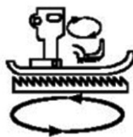
Figure 8: Walking foot of a hand stitch machine
