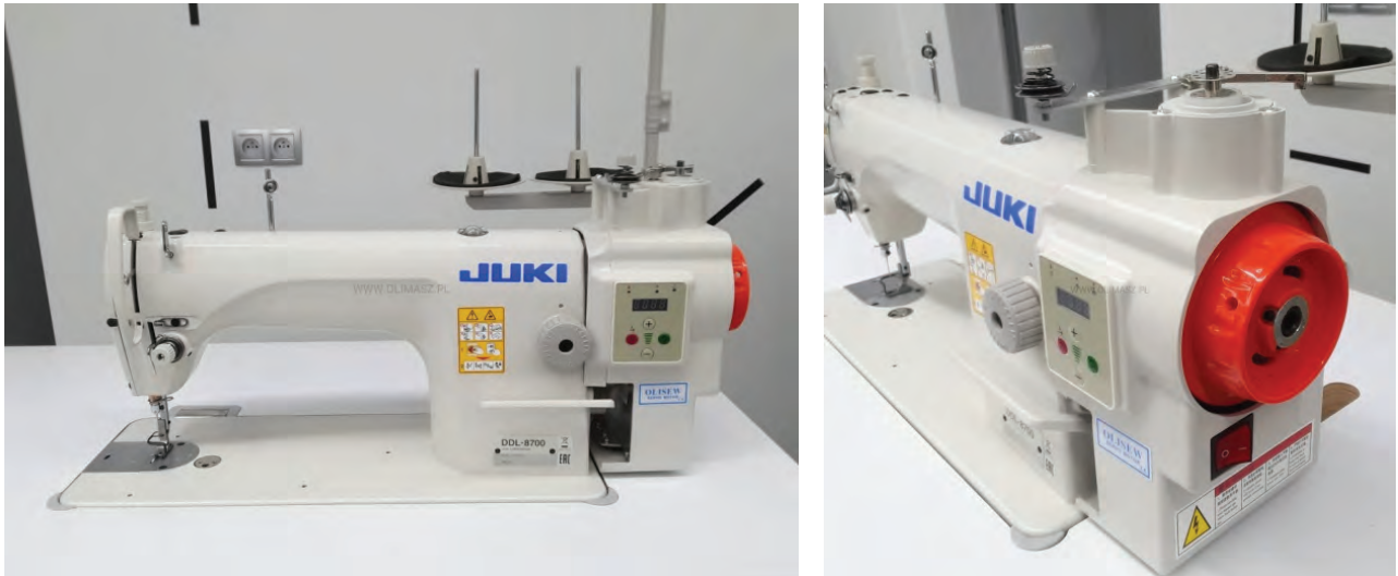
Figure 2: Lockstitch machine JUKI DDL 8700 with Direct Drive motor Slika 2: Motor direktnog pogona na mašine zrnastih uboda JUKI DDL 8700
