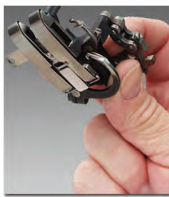
Figure 6: Double side cut presser foot (a) and Presser foot shoes/spacers (b) Slika 6: Obostrani rezač materijala (a) i pritisna nožica sa papučom (b)
