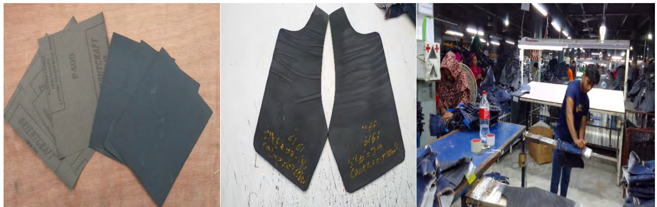
Figure 2: 400 Grade Emery Paper (Left) Rubber Pattern Board (Middle) Manual whisker operation station (Right)
