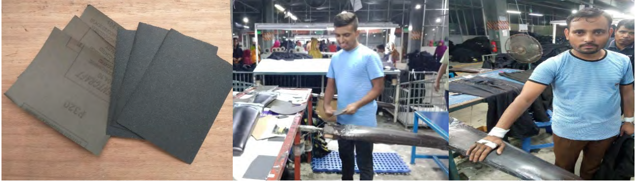
Figure 4: 320 Grade Emery Paper (Left) Manual Scrapping Operation Station (Middle & Right)
