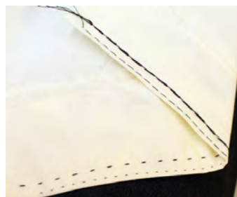
Figure 3: Visual appearance of seams from stitches 209 and 104
