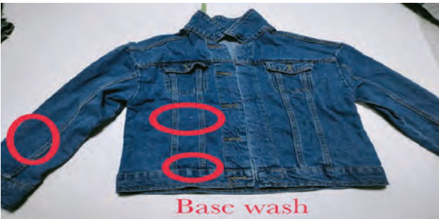
Figure 8: First Wash garments damage issue in case of pumice stone trial
