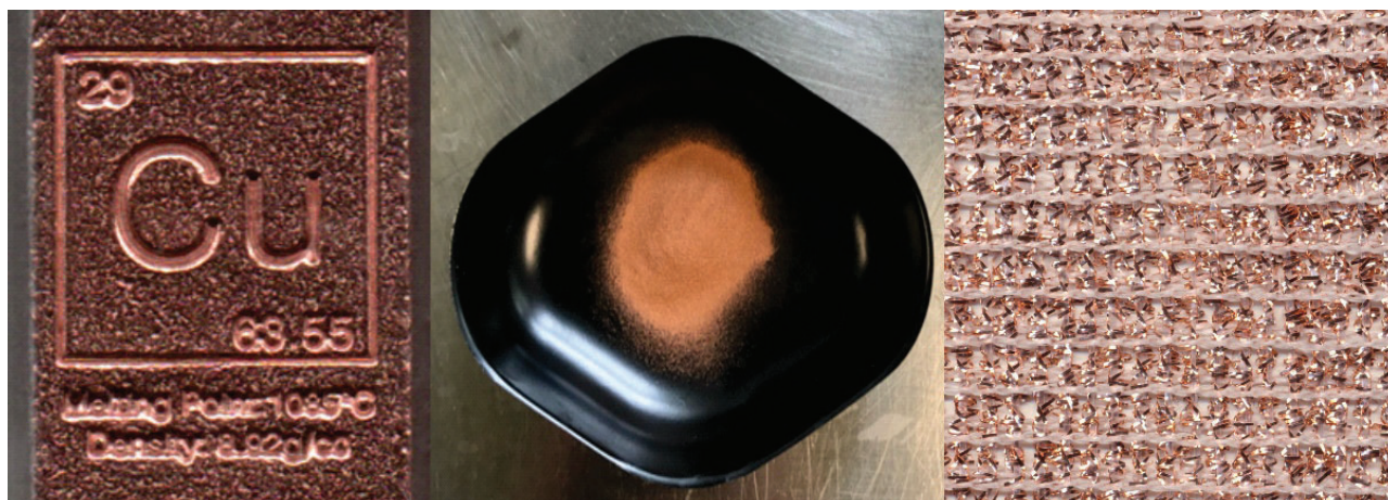
Figure 1: Examples for copper products, from left to right: a metal copper piece, copper pigment powder and a fabric made from polypropylene fibers and copper
