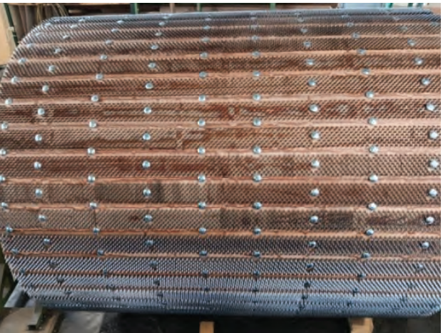
Figure 3: Drums with needles to open textile fibers
