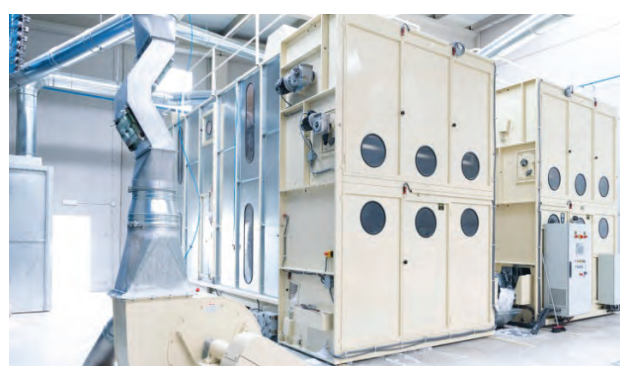
Figure 2: Shredded textile waste blending boxes by company Margasa
