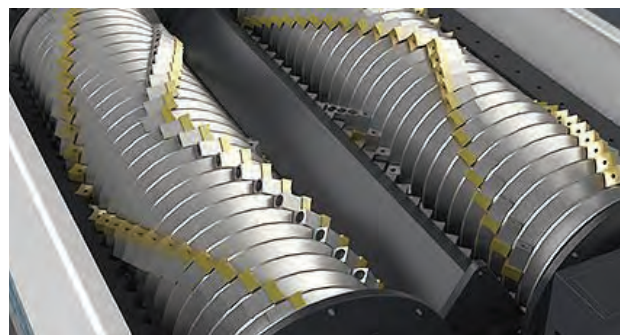
Figure 1: Rotors with knives of the double rotor fine shredder of GSD series by company Gep Ecotech
