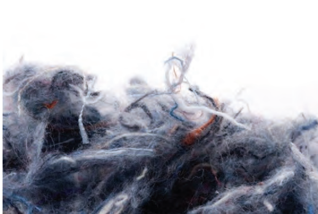
Figure 4: Shredded denim textile waste (a) and fiber tufts after tearing process (b)
