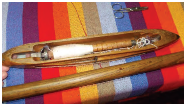
Figure 2: Picking block - shuttle with weft winding
