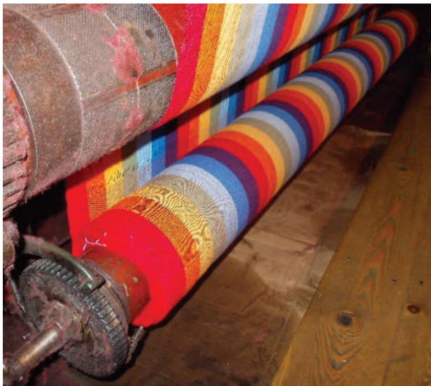
Figure 3: Finished fabric wound on the fabric beam of the Textima loom
