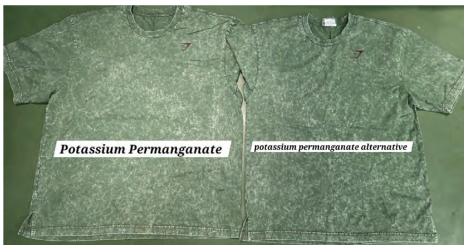
Figure 1: Knit garments after Conventional acid wash with Potassium Permanganate and Acid wash with PP alternative
