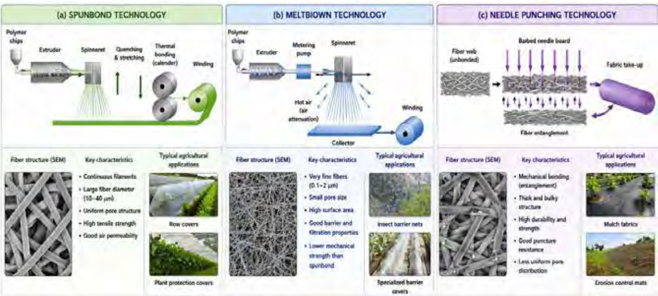
Figure 5: Production technologies for nonwoven agricultural covers and their structure–property–application relationship.
