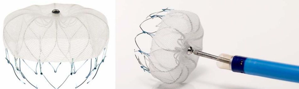
Fig. 3 – Watchman: Left atrial appendage closure device is a nitinol cage with a polytetrafluoroethylene membrane on the surface, and fixation anchors around the perimeter (Courtesy of Boston Scientific).
