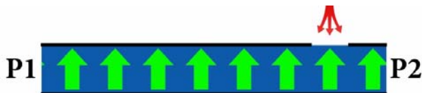
Fig. 8 – During inspiratory part of the positive pressure ventilation, the P_{ins} > P_{atm} , there is a functional sealing of the hole, which prevents the suctioning of the atmospheric air.
