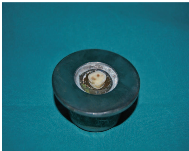
Fig.1 Custom made grinding cylinder.
