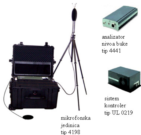
Sl. 1 – Terminal za monitoring buke NMT 3637B
