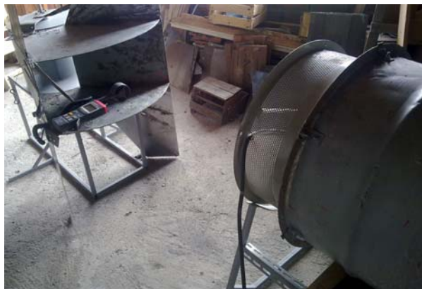
Figure 8 – The process of measuring the wind speed using an anemometer
