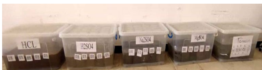
Figure 5 – Acid and sulfate attack test
