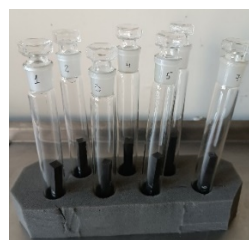
Figure 1 – Left: sample prepared for artificial aging; right: sample prepared for acclimatization in a climate chamber
