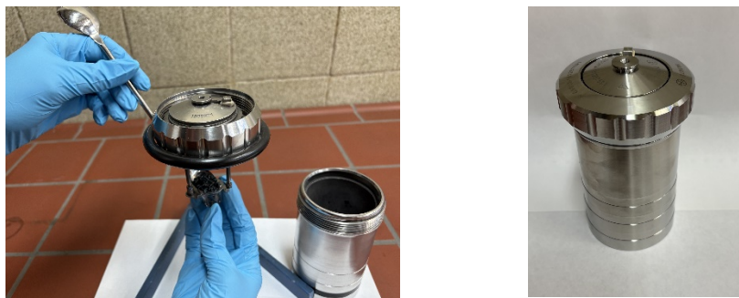
Figure 5 - Left: positioning the sample within the quartz container of the bomb; right: bomb prepared for the experiment
