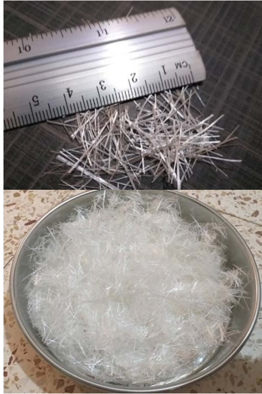
Figure 3 - Glass fibers with a length of 1.50 \pm 0.25 cm
