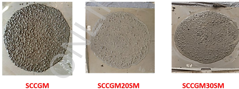
Figure.8 – Visual control of segregation and bleeding of RMA of different SCC mixtures (source author)
