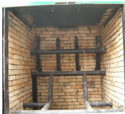
Sl 1 Dvostepena rešetka ložišta kotla termičke snage 300 kW Fig. 1 Twostage grate of firebox boiler with thermic power of 300 kW
