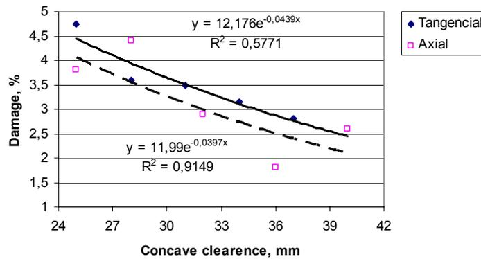
Fig. 2. The effect of the concave clearance on the damage to maize grain
