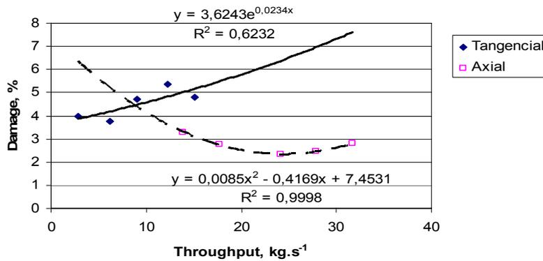
Fig. 3. The effect of the threshing mechanism throughput on grain damage
