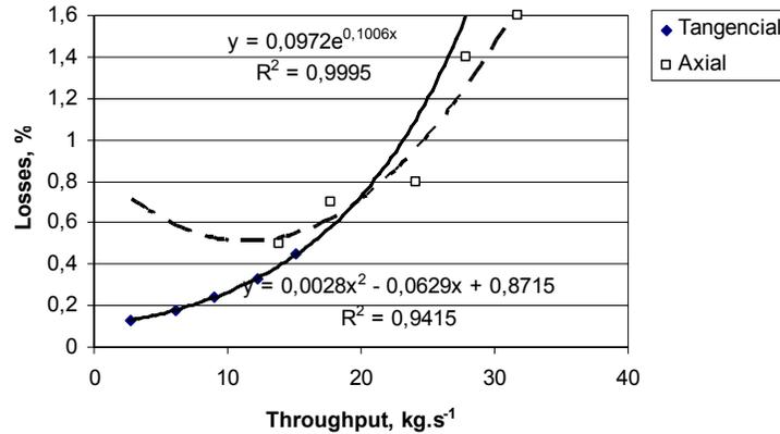
Fig. 6. The effect of combine harvester throughput on the maize grain losses, Axial – cylinder peripheral speed  $12.1 \text{ m.s}^{-1}$ , concave clearance  $32 \text{ mm}$ , grain moisture  $19.2\text{-}28\%$ , Tangential – cylinder peripheral speed  $16.9 \text{ m.s}^{-1}$ , concave clearance  $32/20 \text{ mm}$ , grain moisture  $25\%$
