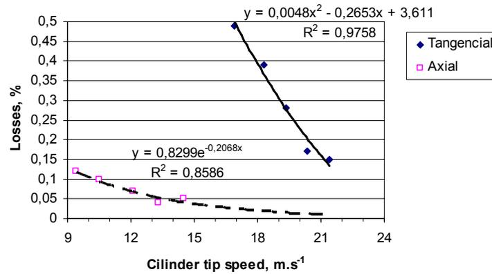
Fig. 4. The effect of the cylinder peripheral speed on the maize grain losses
