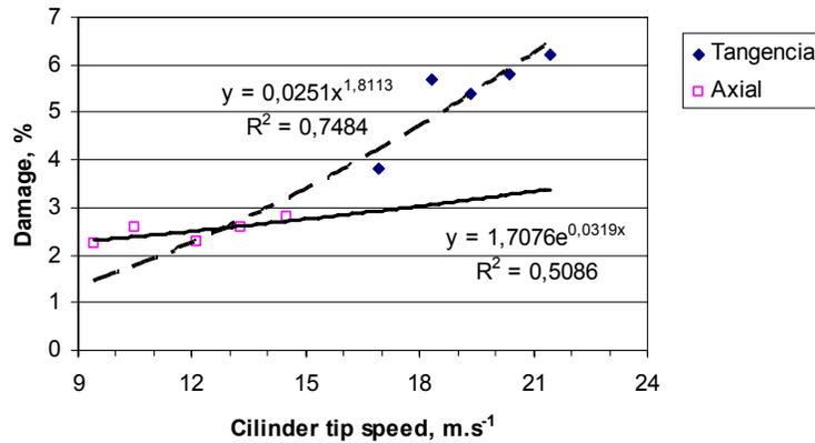
Fig. 1. The effect of the cylinder peripheral speed on the level of damage to maize grain
