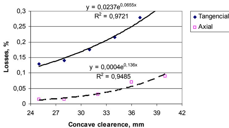
Fig. 5. Effect of concave clearance on the maize grain losses
