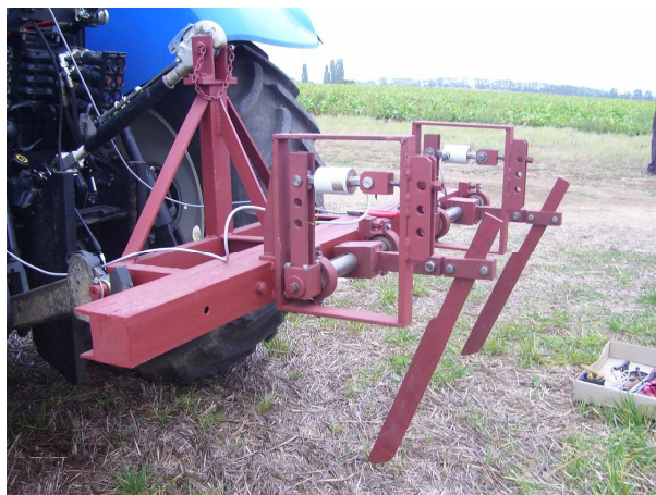
Fig. 5. Horizontal penetration device attached Sl. 5. Prikpočavanje nosača horizontalnog penetrometra
