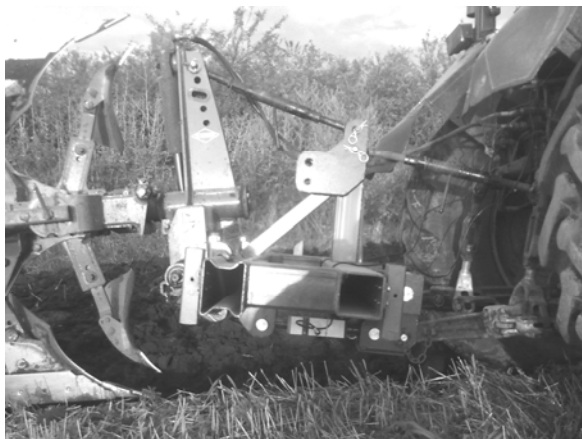
Sl. 6. Univerzalni ram sa plugom na traktoru Fig. 6. Universal frame with plough hitched on the tractor
