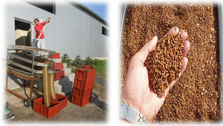
Fig. 1: The separator with planar vibrating sieves Figure 2: The separated seeds vine
