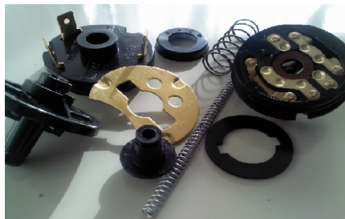
Sl. 7. Sastavni delovi kontakt brave Fig. 7. The constituent elements of the start ignition
